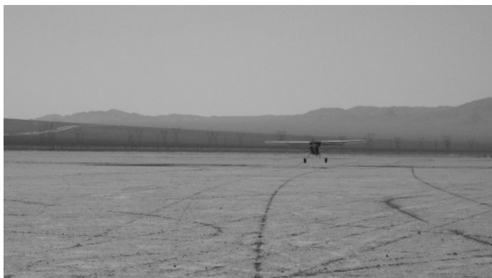
A dry lake bed is used to practice on. By varying the landing direction you can get different degrees of crosswind velocity.
