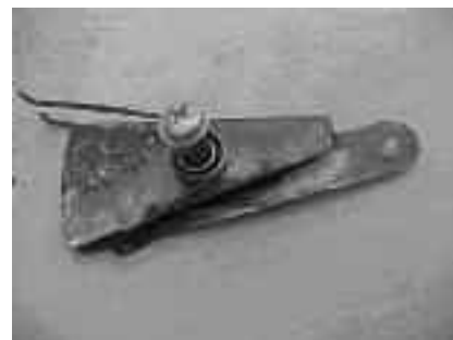
Here is the Latch, removed from the flap lever and showing the MS screw in lieu of aluminum rivet. The hole that operating rod passes thru is on the right. When that hole elongates, or the rod's upset-end loses material due to years of vibration, the rod can disconnect and the flaps will be locked in whatever position they presently are. You will NOT be able to change them in flight. The "trap-spring" is the only spring inside the flap lever and provides all the "feedback" to the release-button.
